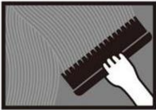
Flooring Installation —Glue coating
